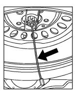
2. If the cable is visible, place the wrench on the hoist drive nut and turn the wrench counterclockwise until approximately 6 inches (15 cm) of cable is exposed.
